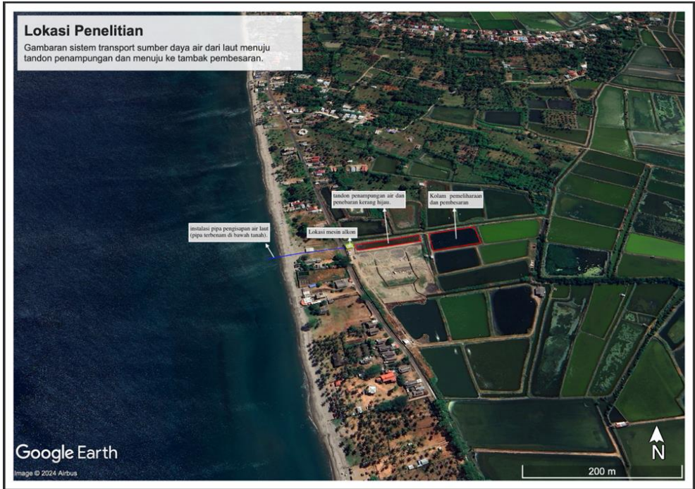
Figure 1. Research Location and Overview of the Water Resource Transportation System from the Sea to the Reservoir and to the Grow-Out Pond
